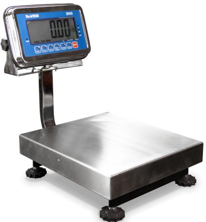
The WorldWEIGH C300 Series Bench Scale is an economical yet robust choice for basic weighing and parts counting. Arriving fully calibrated and ready for use, it supports capacities up to 250 lbs. It features a stainless steel weighing platform, a durable carbon steel base, and includes a stainless steel indicator. Additionally, it offers NTEP approval, ensuring precise and trusted measurements for various industrial applications.
