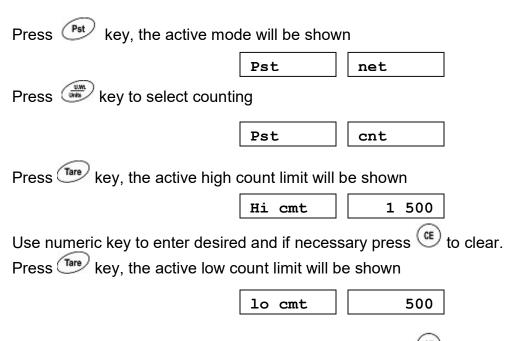
Use numeric key to enter desired and if necessary press  $\textcircled{\text{CE}}$  to clear. Press  $\textcircled{\text{Tare}}$  key to return weighing mode.
